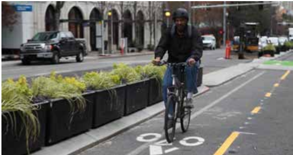
Two-Way Protected Bike Lane with Planters
