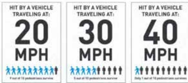
Nine out of 10 people walking survive when hit by a vehicle traveling at 20 MPH, but only five do when hit at 30 MPH and only one when hit at 40 MPH. US DOT NHTSA (1999)
