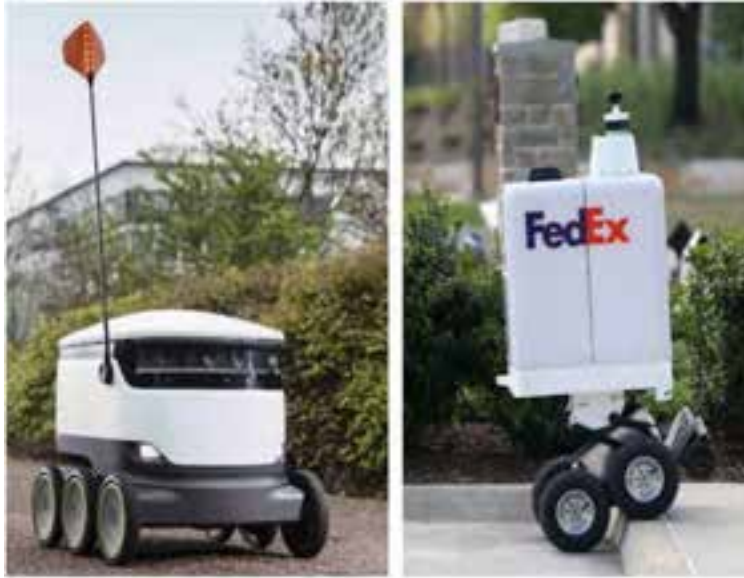
A Starship Personal Delivery Devices (PDD and a FedEx Delivery Robot making autonomous deliveries. Image Source: http://www.dot.state.mn.us/automated/docs/personal-delivery-device-white-paper.pdf
