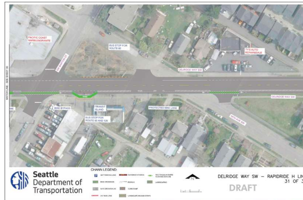
30% Street Design Channelization Plan
