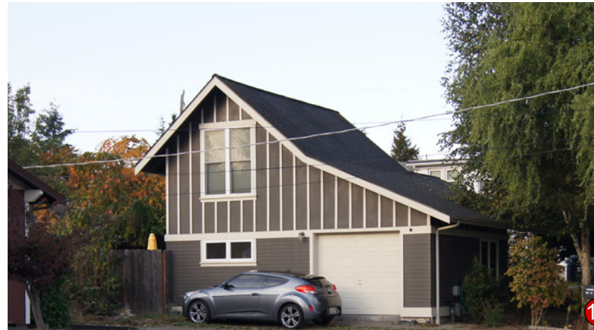
Board and Batten Facade; Two Part Composition;
